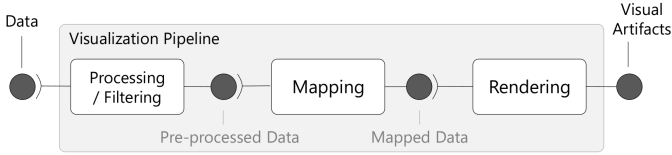
Fig. 3. Model of a visualization pipeline: First, the raw data is undertaken through pre-processing and filtering; second, the pre-processed data is mapped to a geometrical representation; third, the geometrical representation is rendered as an image [16].
